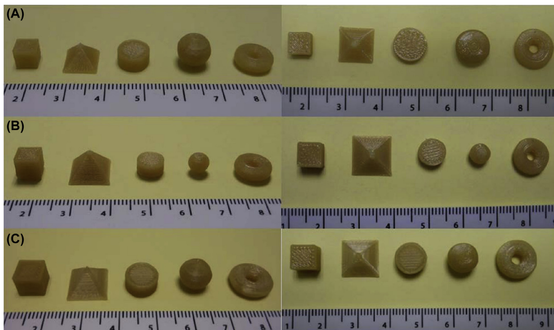
FIGURE 2.9 3D-printed dosage forms of various geometries using poly(lactide) as the primary matrix for tunable release rates at constant (A) surface area, (B) surface area/volume ratio, and (C) mass (scale bar in cm). Adapted from Goyanes A, Chang H, Sedoug HD, Hatton GB, Wang J, Buanz A, Gaisford S, Basit AW. Fabrication of controlled-release budesonide tablets via desktop (FDM) 3D printing. Int J Pharm 2015b;496:414–420; Goyanes A, Martinez PR, Buanz A, Basit AW, Gaisford S. Effect of geometry on drug release from 3D printed tablets. Int J Pharm 2015c;494:657–663; Goyanes A, Buanz AB, Hatton GB, Gaisford S, Basit AW. 3D printing of modified-release aminosalicilate (4-ASA and 5-ASA) tablets. Eur J Pharm Biopharm 2015a;89:157–162; Goyanes A, Wang J, Buanz A, Martínez-Pacheco R, Telford R, Gaisford S, Basit AW. 3D printing of medicines: engineering novel oral devices with unique design and drug release characteristics. Mol Pharm 2015d;12:4077–4084.
